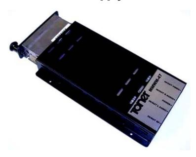
The MMWM-47 is a stand alone chassis designed to hold any of the industries minimod type headend pieces such as a modulator, demodulator, stereo encoder, converter or digital demodulator. The MMWM-47 is ideally suited for wall mounting, using on an A/V cart, or mounting to the back of a TV/monitor. The chassis has four 1/8" diameter mounting holes along the flanges and ventilation slots on the sides for heat dissipation. It comes with a universal power supply for domestic and international use.
